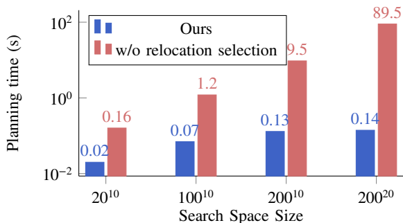
Fig. 5: Planning time (in log scale) with respect to search space size for planning robot contacts for cube sliding. We have search\ space\ size = candidate\ contacts^{trajectory\ size} .
